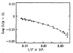
Fig. 4.—The probability of quenching per encounter as a function of temperature.
