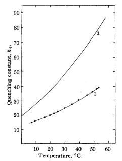
Fig. 3.-The calculated encounter rate (1), and the experimental quenching constant (2) as a function of temperature.
